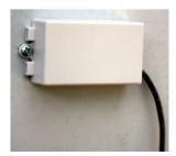
**Outdoor Sensor (OT)** – extend sensor to an outdoor location properly sampling the outdoor temperature. Select a location away from direct sunlight and where the sensor will not pick up false temperature from the heat pump outdoor unit, refrigerant line sets, dryer vent, reflection off of steel siding, etc. Do not install the sensor in any type of enclosure, as this will falsely trap and pick up radiant sun temperature. Mount the sensor horizontally on the structure using the screws provided.
