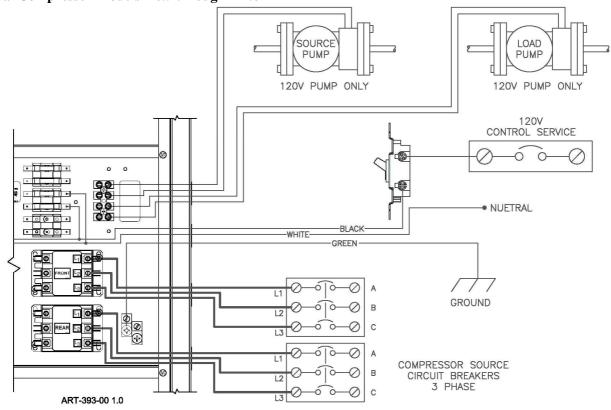
**Note**: Some local codes and CEC electric code may require single disconnect and single feed for the main compressor power source. If this is the case, the installer must provide disconnect with multi-feeds per above.
